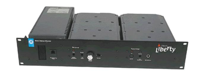
The new T800SL range of base stations provides high-end base station performance at a low-end price. Using proven T800 modules as an RF platform, professional 25W base-station performance is obtainable at similar prices to that of two mobiles in a box.
